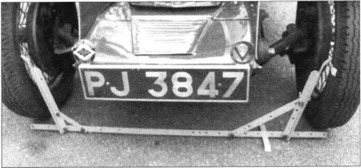
Figure 3 Gauge in position in front of the axle.
