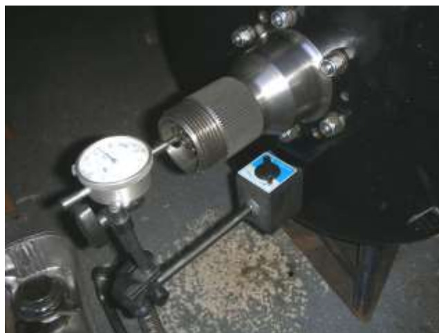
Measuring the axial clearance
