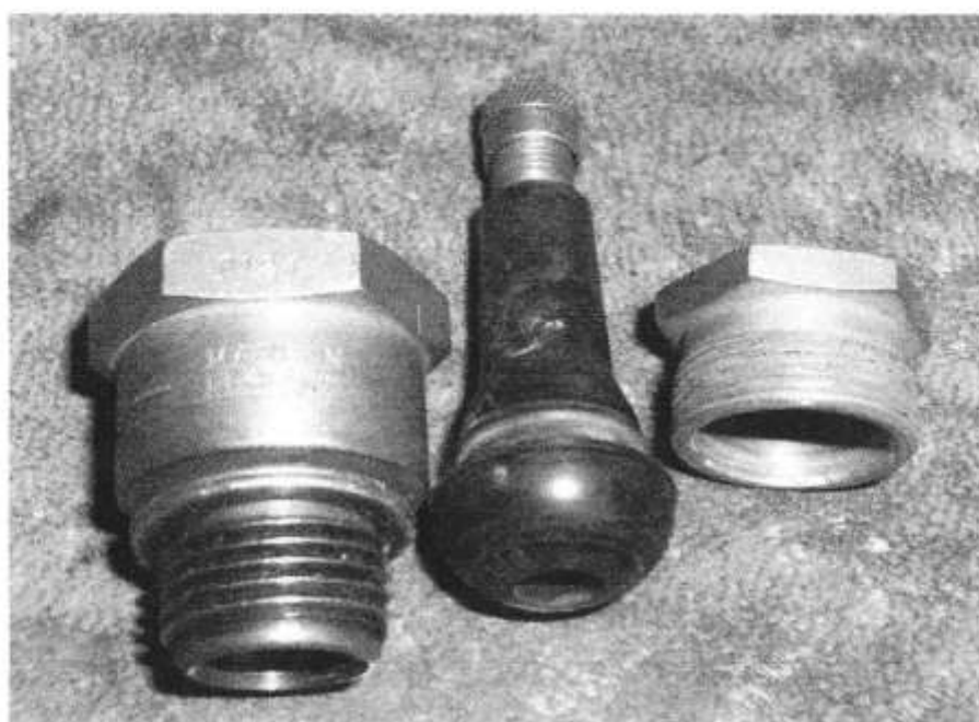
Above: The components of the air plug .
