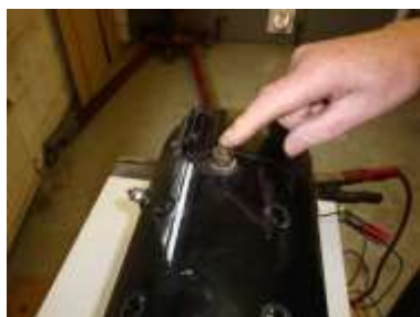
The main terminal at front of dynamotor. This receives 24v in start mode on 21hp cars
