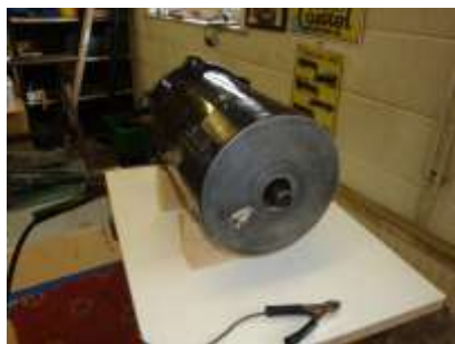
The front face of dynamotor showing removable brush cover
