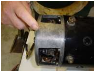
Refit band so join is on a solid face
