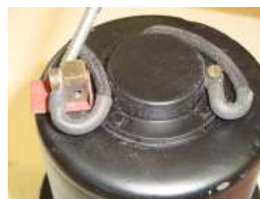
Solenoid terminal on left. Earth on right. Make sure both are tight
