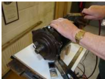
Test starting with positive to the main terminal
