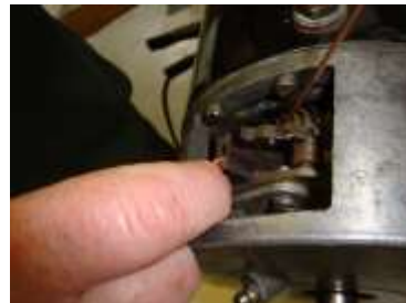
Spring held back and brush being eased out of holder
