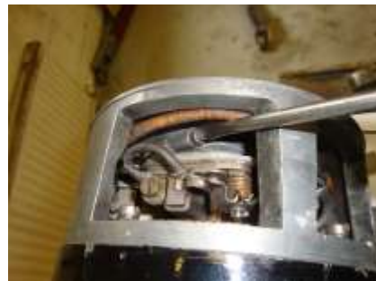
Slacken fifth brush screw and move ring in small increments
