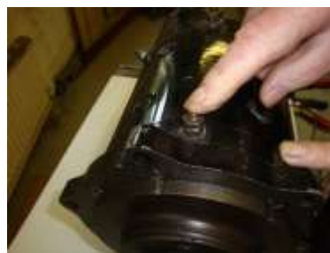
The field terminal at rear of dynamotor. This is always at 12v on all cars
