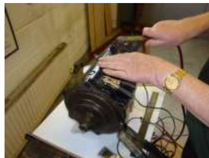
Test charging by connecting field and main terminals
