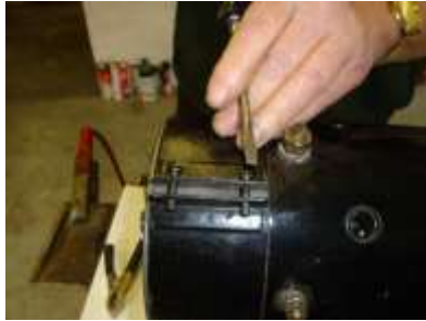
Access brush gear by undoing two screws and sliding steel band forward
