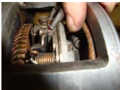
Inner screw adjusts main brush holder. Outer screw adjusts fifth brush
