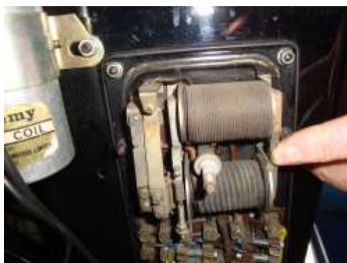
The twin coil relay. Charging contacts on the left, solenoid on the right
