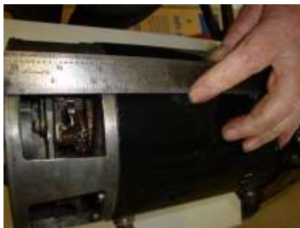
Set edge of brush holder in line with bolt centres
