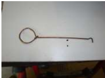
Improved hook to pull back brush retaining springs
