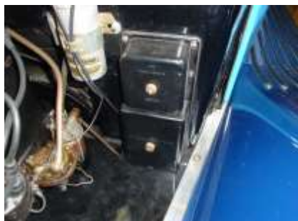
The cut out above and fuse box below
