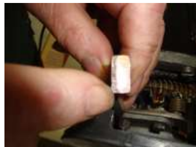
Spring held back and brush being eased out of holder
