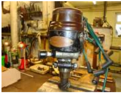
The distributor showing cap and leads. Condenser is under distributor body. Greaser on the left
