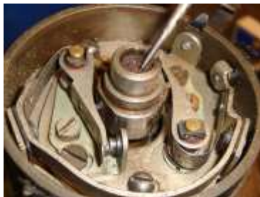
Rotor arm removed showing felt pad. Oil sparingly from time to time
