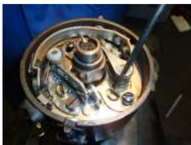
Adjust by rotating eccentric screw
