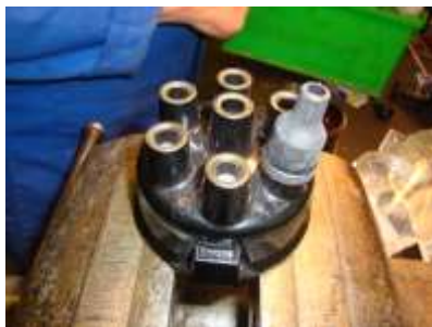
Modern distributor cap with push in leads
