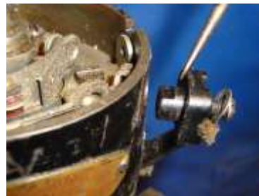
Remove base plate by removing two spring clip screws
