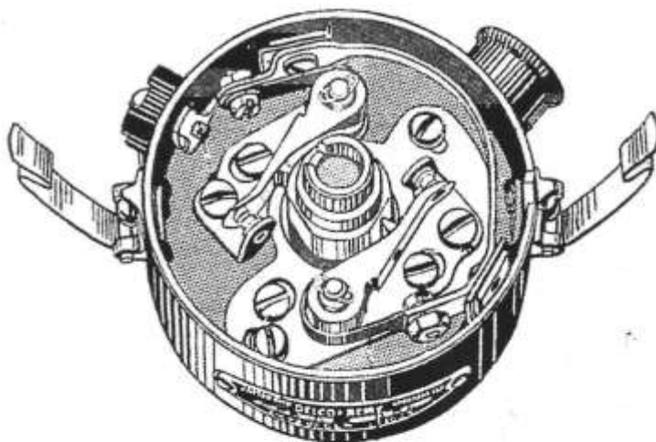
Above: The dual contact breakers fitted to 6 cylinder Talbot cars.
