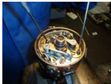
Slacken base plate retaining screws prior to adjustment.
