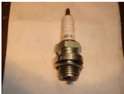
The correct NGK plug: AB6 (gap to 25 thou)
