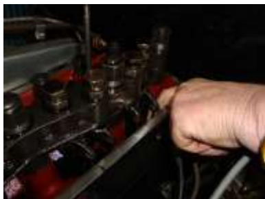
Checking TDC at the valves. Inlet and exhaust pushrods rotate
