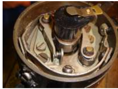
Cap removed showing rotor arm, cam and twin points
