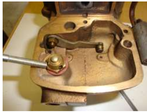
Needle valve. Fuel level is adjusted by changing the fibre washer
