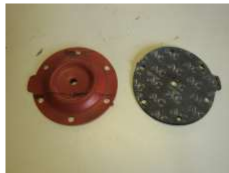
New diaphragm on right. Will need to be un-riveted from its rod
