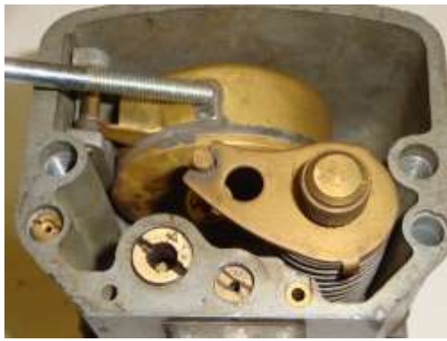
Float and accelerator pump in bowl. Slow running jet on the right
