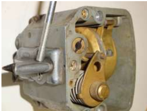
Emulsion tube which projects into venturi
