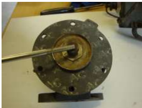
The original diaphragm held by a nut
