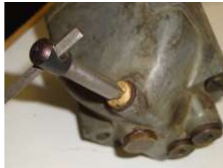
Removing economy jet blanking plug
