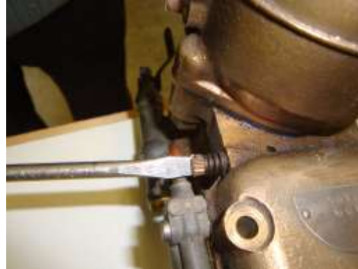
Slow running mixture controlled by air bleed screw
