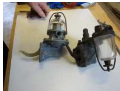
Later AC pumps can be fitted but will need a modified lever
