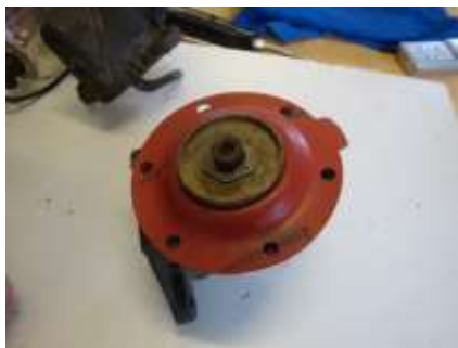
New diaphragm fitted
