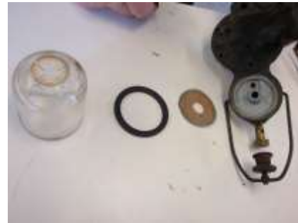
Glass bowl and gauze filter should be removed and cleaned annually
