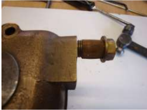
Remove gauze filter from petrol pipe union and swill in clean petrol
