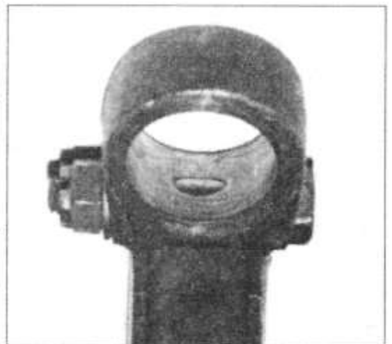
Above: Talbot con rod showing the cotter pin for securing the gudgeon pin.
