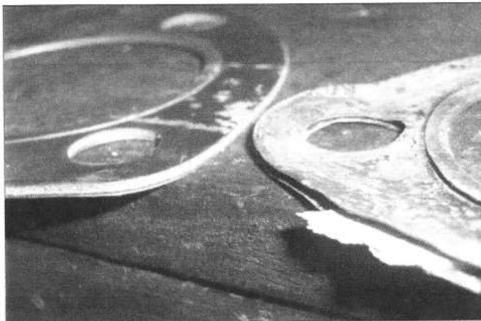
Fig.8 - New copper/asbestos substitute sandwich type manifold/exhaust pipe gaskets before and after 500 miles use.
