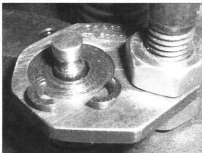
Above: The tool shown over the valve allowing the collets to be removed.
