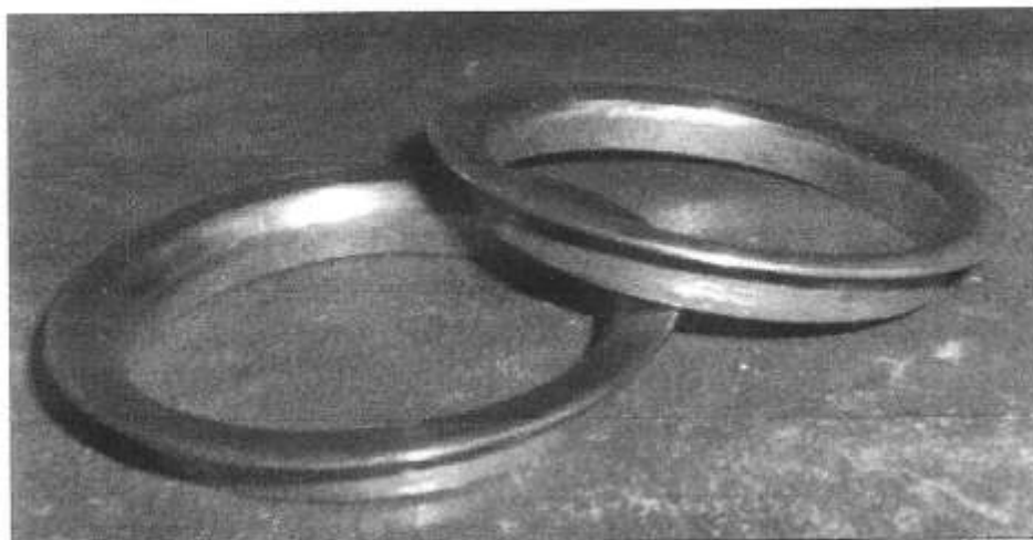
Fig.9 - Solid copper manifold/exhaust pipe gaskets spun from 16 gauge copper tube.
